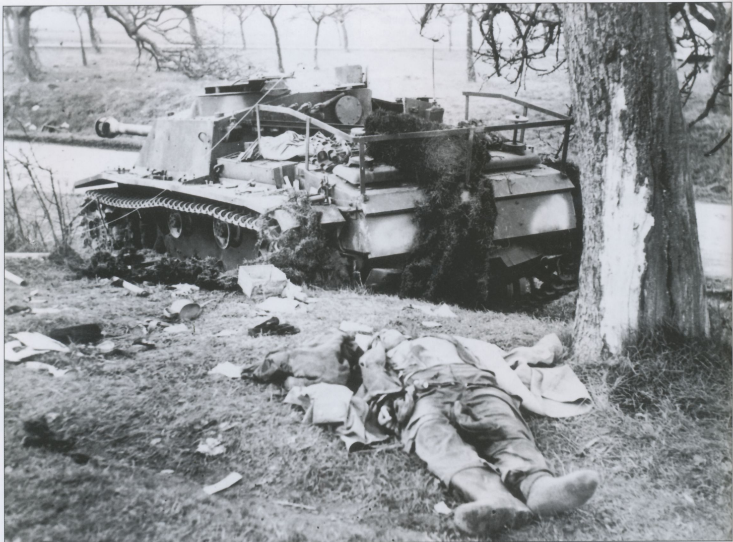
A knocked out late StuG.III Ausf.G somewhere in Western Europe in the late fall of 1944 or early spring of 1945. The vehicle has taken a hit, low in the left side, which has blown off the first return roller and damaged the drive sprocket. It appears that part of the rear plate of the fighting compartment behind the loader, has been neatly cut out for some unknown reason.
