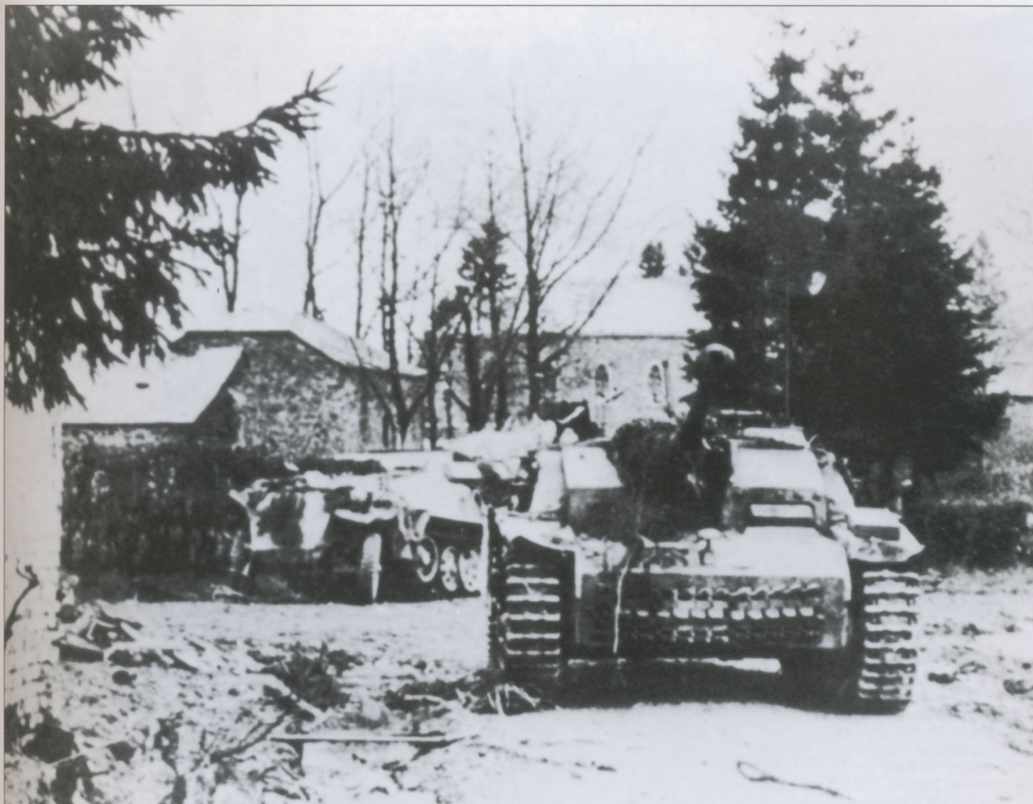
A StuG.III Ausf.G and an Sd.Kfz.251/1 Ausf.D sit abandoned near Manhay, Belgium in late December 1944. This is a late production StuG.III without Zimmerit and equipped with the remote control machine gun mount on the fighting compartment roof, 80mm front plate on the right side of the superstructure, barrel travel support and deflector in front of the commander's cupola.
