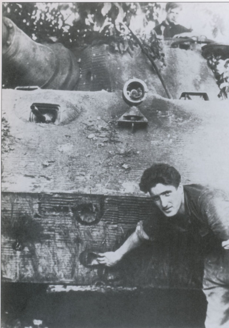
A crewman from s.Pz.Abt.503 points out the punishment absorbed by the 100mm thick, sloped armor plates of the Tiger II that resulted only in deep gouges and chipped Zimmerit coating, but did not otherwise cause any damage.
