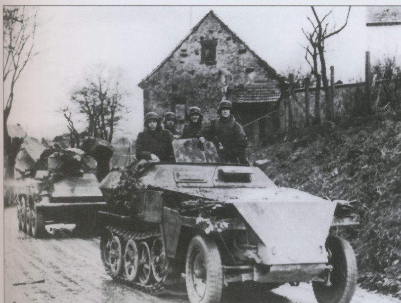
An Sd.Kfz.250/1 (Neu) followed by an Sd.Kfz.234/3 from 116.Panzer-Division pass through a German village near Aachen in the fall of 1944. The Sd.Kfz.234/3 mounted the 7.5cm KwK51 L/24 and were issued to the reconnaissance companies of the Panzer divisions to provide anti-tank support. A total of 88 were produced from June to December 1944.
