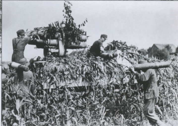
The 15cm Nebelwerfer 42 projectiles weighed 34 kilograms and had a range of 6,900 meters. The rockets were not very accurate and the Germans relied on blanketing the area with a heavy concentration of fire. Armored vehicles were practically immune to all but a direct hit but unprotected infantry were more susceptible to the explosive force of the blast, the thin casings providing little in the way of fragmentation.
