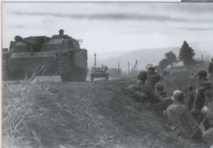
A StuG.III Ausf.G passes an infantry squad huddled in a ditch in Rumania in late October 1944. The Schürzen have been field modified to hang on short pieces of pipe welded to the fenders. The plates were held in place with a cotter pin that allowed them to rotate freely when traveling through dense brush and which prevented them from being torn off and lost. A single or sometimes double plate was fixed on the side of the fighting compartment to protect the upper sides.
