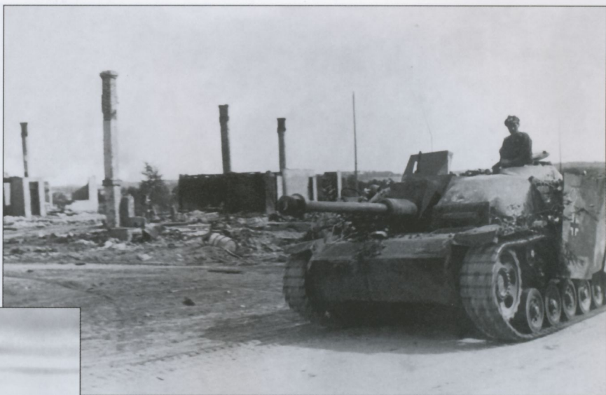
A StuG.III Ausf.G passes an infantry squad huddled in a ditch in Rumania in late October 1944. The Schürzen have been field modified to hang on short pieces of pipe welded to the fenders. The plates were held in place with a cotter pin that allowed them to rotate freely when traveling through dense brush and which prevented them from being torn off and lost. A single or sometimes double plate was fixed on the side of the fighting compartment to protect the upper sides.
