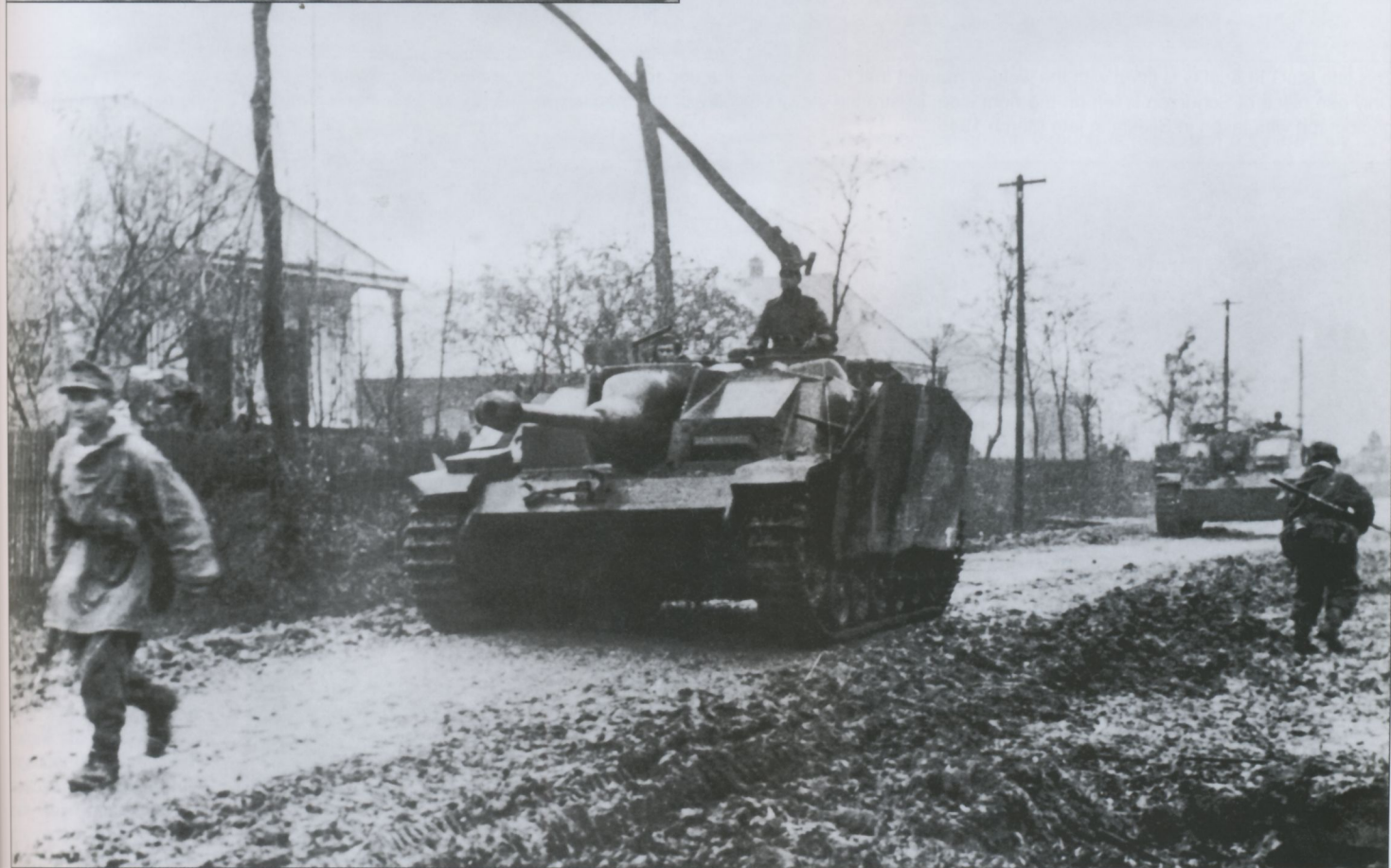
This late production StuG.III Ausf.G was manufactured after September 1944 when the application of Zimmerit was discontinued. It is also fitted with the folding gun travel lock on the glacis and single 80mm thick plate on the right side of the superstructure, which were introduced in July 1944. The remote MG mount, or Rundumfeuer, was introduced in April 1944 but shortages of the weapon meant that there were many vehicles issued without them. The loader's hatches were redesigned to open to the sides to accommodate the device, which could be operated with safety from inside the vehicle using a periscopic sight.
