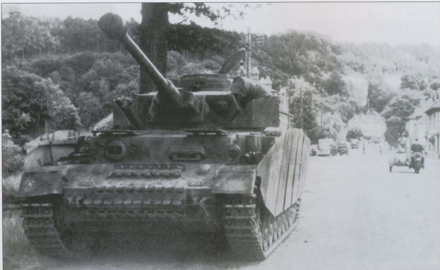
A new Pz.Bef.Wg.IV Ausf.H parked alongside a road on the way to the invasion front. A 2m 'Sternantenne D' (star antenna) for the Fu 8 radio set can be seen mounted where the normal antenna was mounted which, along with the lack of a tactical number on the turret skirt, would indicate this is probably a II.Bataillon command vehicle. Production of the Pz.Bef.Wg.IV. started in March 1944 with 88 units being converted from rebuilt Panzer IV's. Records indicate that the division was issued with 5 on 30 April 1944. The divisional emblem of the 12.SS-Panzer-Division can be seen painted in white on the right mudguard.
