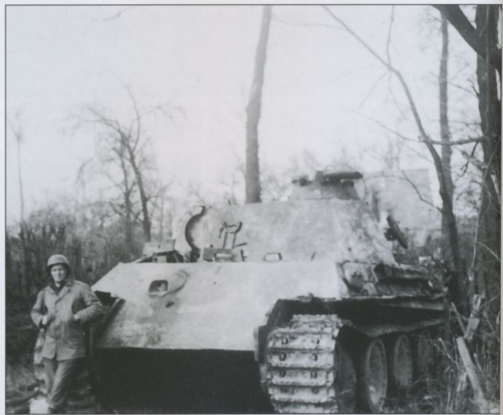
Another derelict Panther Ausf.G photographed near Almen, Germany in 1945. This Panther is fitted with the reinforced chin mantlet and appears to be missing its gun barrel. Two faint numbers, '37', can be seen on the side of the turret.
