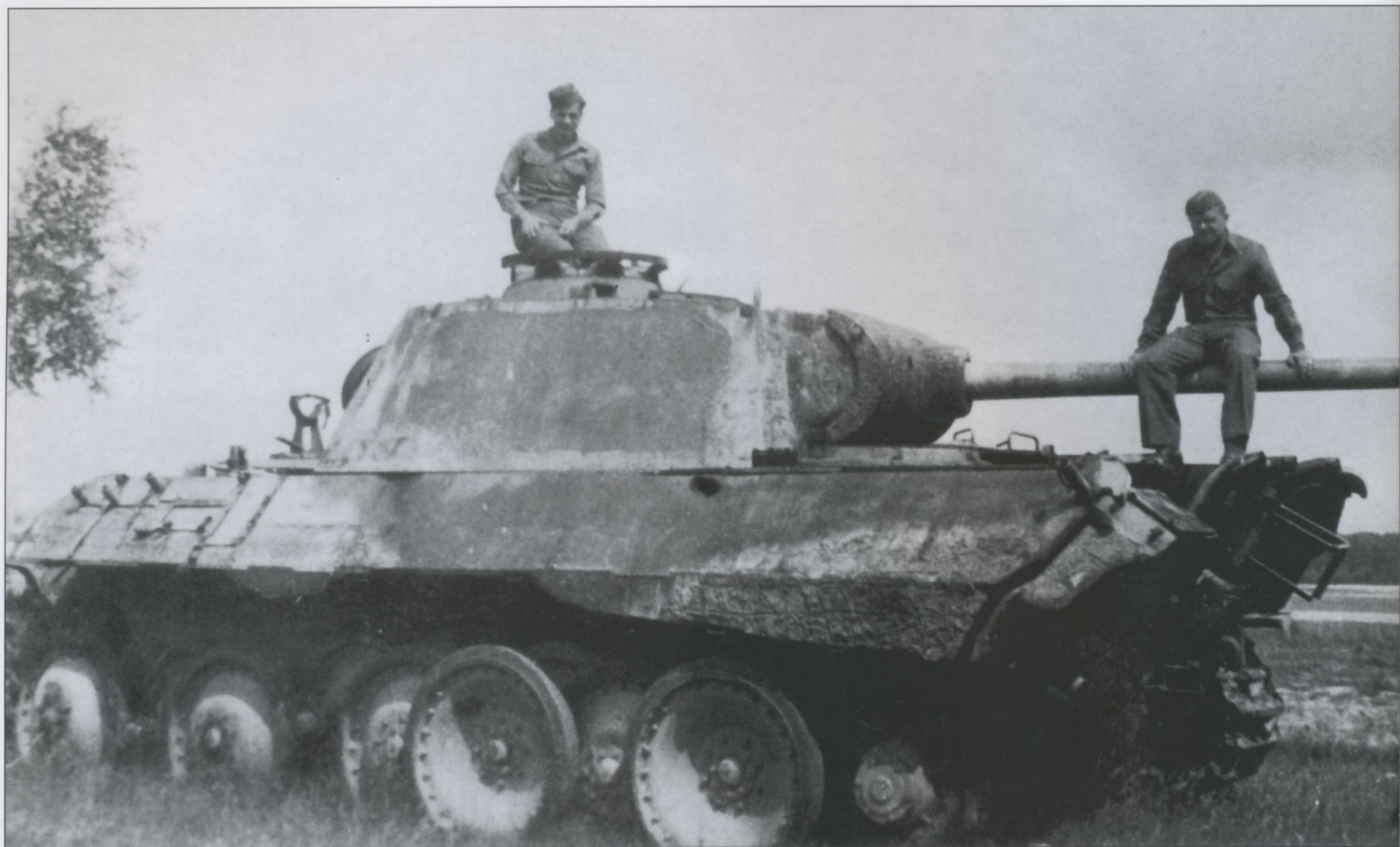
Two U.S. servicemen pose with a Panther Ausf.A near Braunschweig, Germany in early 1945. The penetration hole from the shot that knocked it out can be seen just below the top of the engine deck. The resulting fire has burned away the Zimmerit coating on part of the hull and side of the turret.
