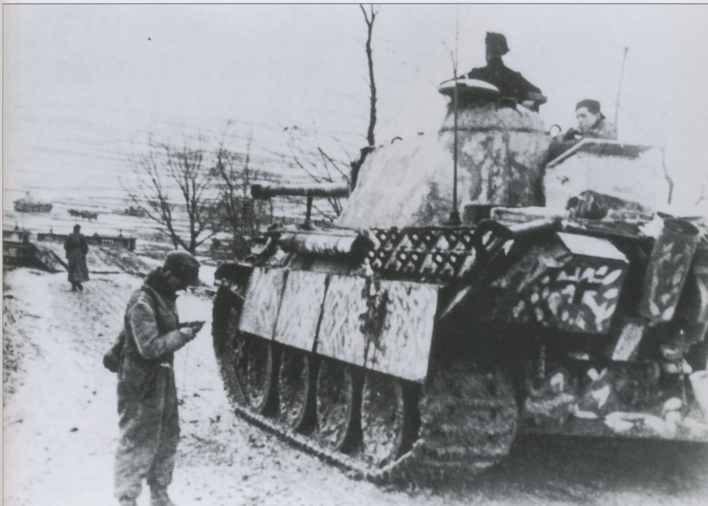
A Panther Ausf.G from I./SS-Pz.Rgt.1 of 1.SS-Panzer-Division 'LSSAH' photographed in the Gran bridgehead area of Hungary during Operation Südwind in late February or early March 1945. The Panther is fitted with the vertical 'Flammenvernichter' flame dampening exhaust and raised cooling fan tower used to provide heat to the crew compartment in cold weather.
