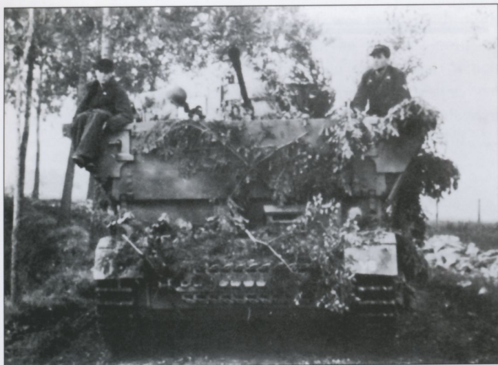
The Flakpanzer IV 'Möbelwagen' was armed with the 3.7cm Flak 43 mounted on a Pz.Kpfw.IV Ausf.J chassis. The first twenty units were completed in March 1944 and the following June, eight were issued to each of the 9., 11. and 116.Panzer-Divisions in the west. A total of 240 units were produced by March 1945.
