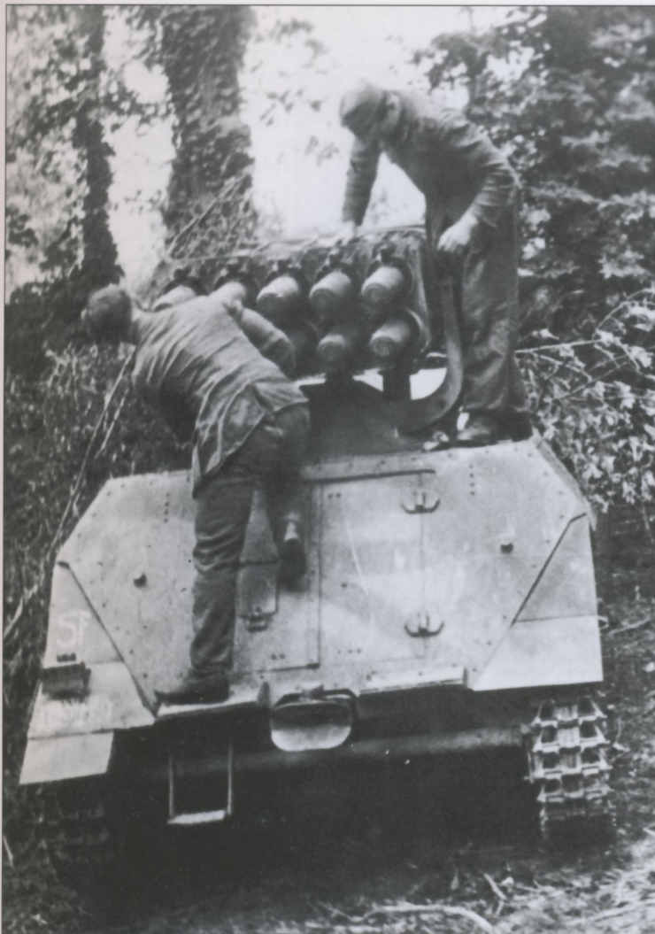
The 15cm Nebelwerfer 42 projectiles weighed 34 kilograms and had a range of 6,900 meters. The rockets were not very accurate and the Germans relied on blanketing the area with a heavy concentration of fire. Armored vehicles were practically immune to all but a direct hit but unprotected infantry were more susceptible to the explosive force of the blast, the thin casings providing little in the way of fragmentation.
