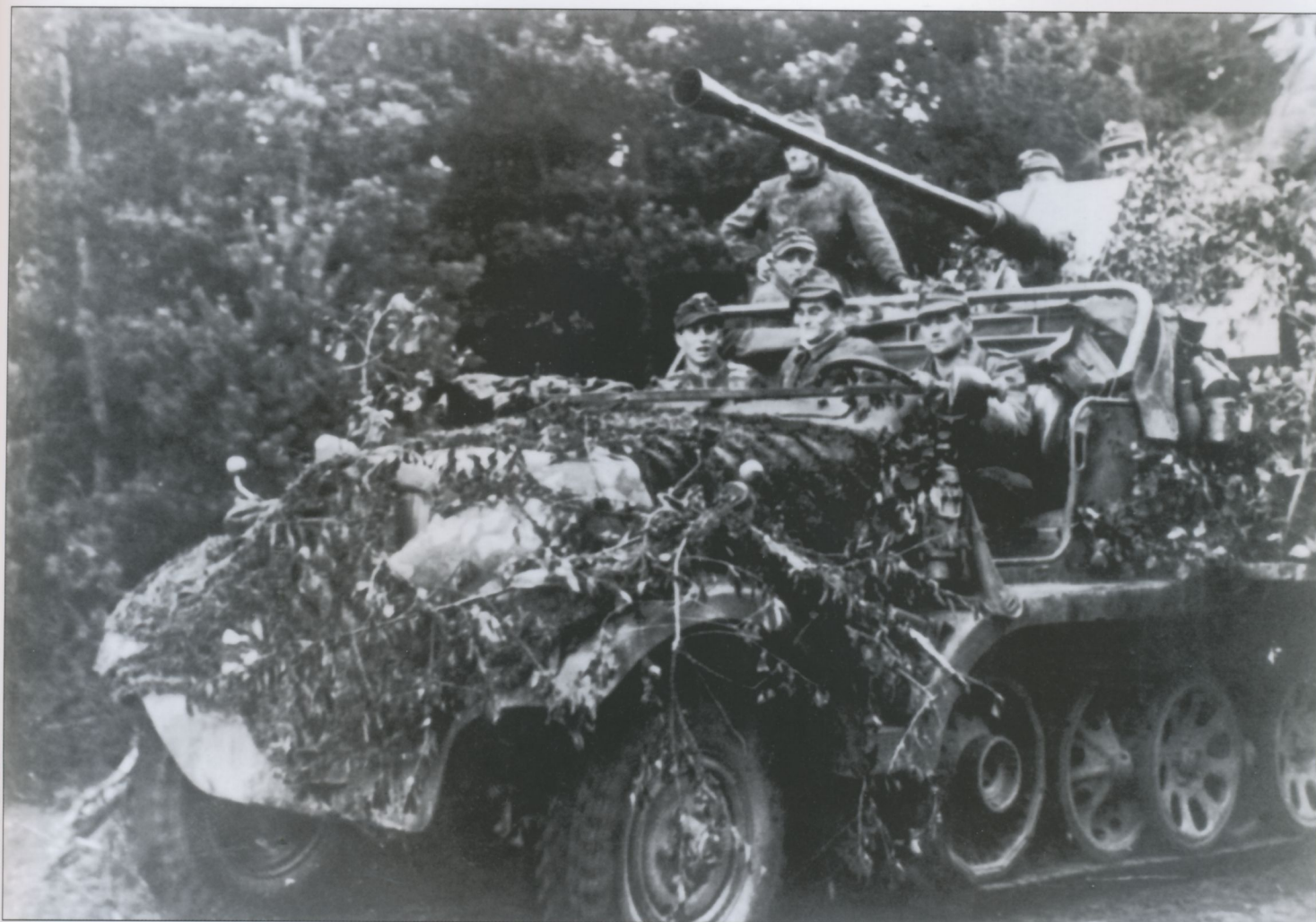
The Sd.Kfz.6/2 carried the 3.7cm Flak 36, which had a practical rate of fire of 80-100 rounds per minute. Although this was slower than the 2cm Flak, it had a horizontal range of 6600 meters and a ceiling of 4800 meters. The Sd.Kfz.6/2 were issued almost exclusively to Luftwaffe Flak Regiments, the exception being 18 issued to Regiment 'Großdeutschland'.
