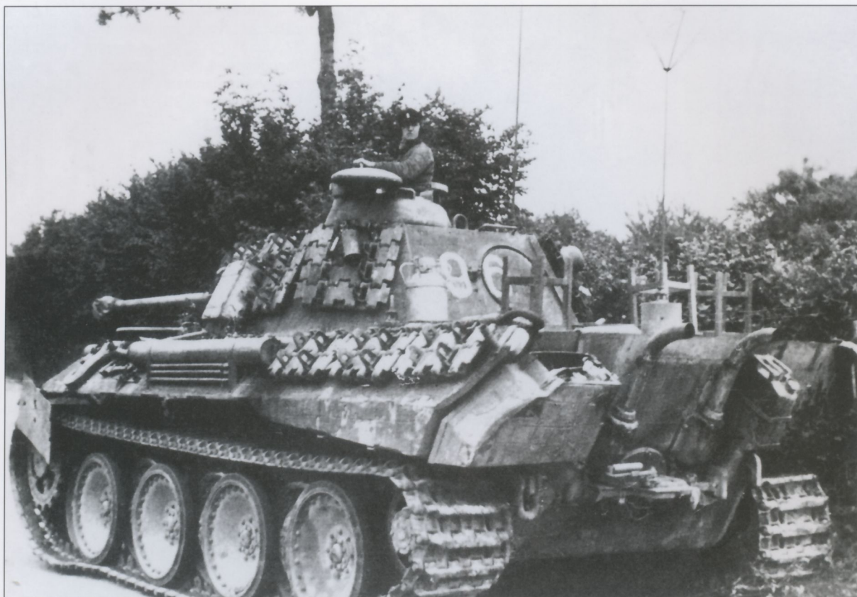
A Panzerbefehlswagen V Panther Ausf.A from II./Pz.Rgt.33 of 9.Panzer-Division in Normandy. The division suffered heavy losses on its journey to the invasion front and served for only about two weeks at the beginning of August. Judging from the battle scarred condition of this vehicle, it was involved in some intense fighting. This is an early production Ausf.A as indicated by the horizontal jack mount.
