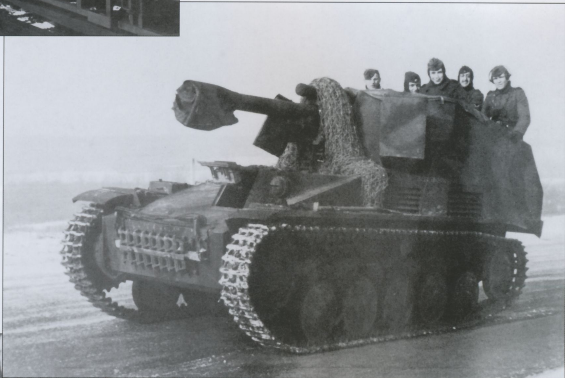
Three photos of 'Wespe' self-propelled light field howitzers of SS-Pz.Art.Rgt.10 from 10.SS-Panzer-Division 'Fruindsberg' while they were stationed in France during the winter of 1943-44. Built on the modified chassis of the Pz.Kpfw.II, the 'Wespe' mounted the 10.5cm leFH18/2 and were issued to the Panzer-Artillerie-Regiments of the Panzer and Panzer-Grenadier divisions.
