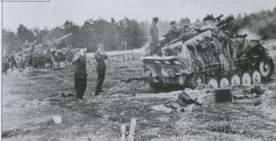
A battery of Wespe self-propelled howitzers fires on enemy positions in the Soviet Union in August 1944. The Wespe carried the 10.5cm leFH18M gun mounted on a modified Pz.Kpfw.II chassis and had a crew of 5 men. They were issued to the Panzer-Artillerie-Regiments of the Panzer and Panzer-Grenadier-Divisions and first saw action at Kursk in July 1943.
