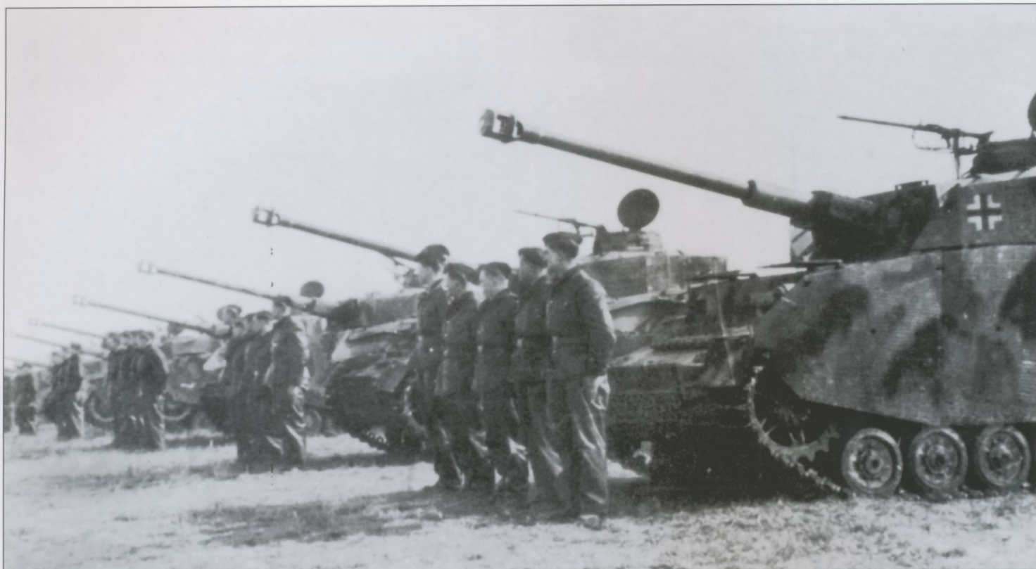
The crews from 5.Kompanie of II./SS-Pz.Rgt.12 from 12.SS-Panzer-Division 'Hitlerjugend', line up in front of their new Pz.Kpfw.IV Ausf.H for inspection. The vehicles are painted in Dunkelgelb RAL 7028 with a camouflage scheme of Rotbraun RAL 8017 and Olivgrün RAL 6003 patches sprayed randomly over the Zimmerit anti-magnetic mine paste. At this time, the three digit tactical numbers were painted in a black-stenciled outline. The crewmen are wearing the black leather U-Boat jacket and trousers, which had been originally provided to the Italian Navy and were brought back to Germany by 1.SS-Panzer-Division 'Leibstandarte' in the fall of 1943.
