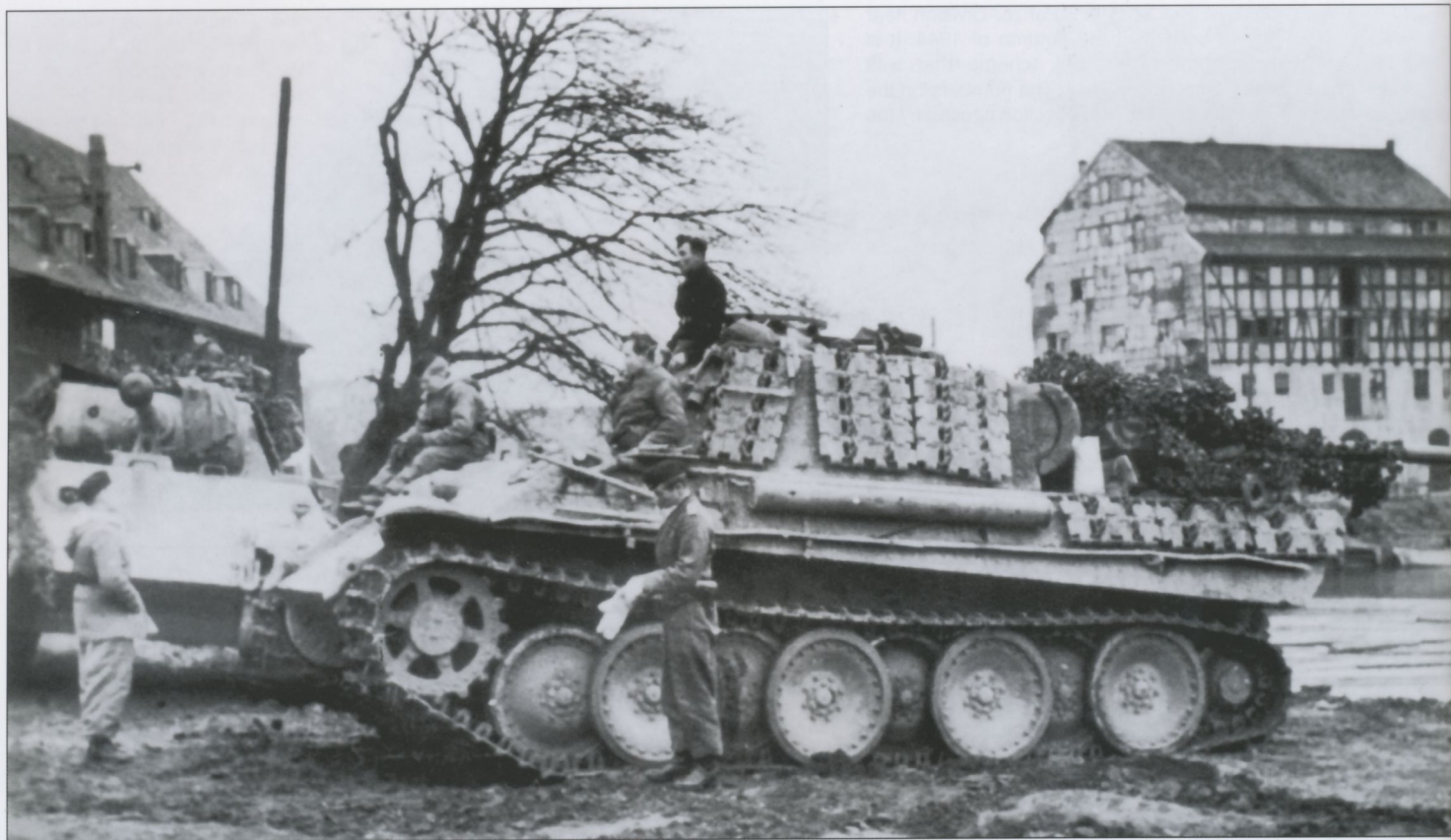
A Panther Ausf.G from an unknown Army unit, photographed after arriving at the Baltic port of Memel, Lithuania in early December 1944. Telltale signs of previous battles can be seen in the form of shrapnel holes in the gun cleaning rod storage tube mounted on the side of the tank. Russian forces surrounded the port in October 1944 and strong German resistance prevented them from taking the city until 27 January 1945.
