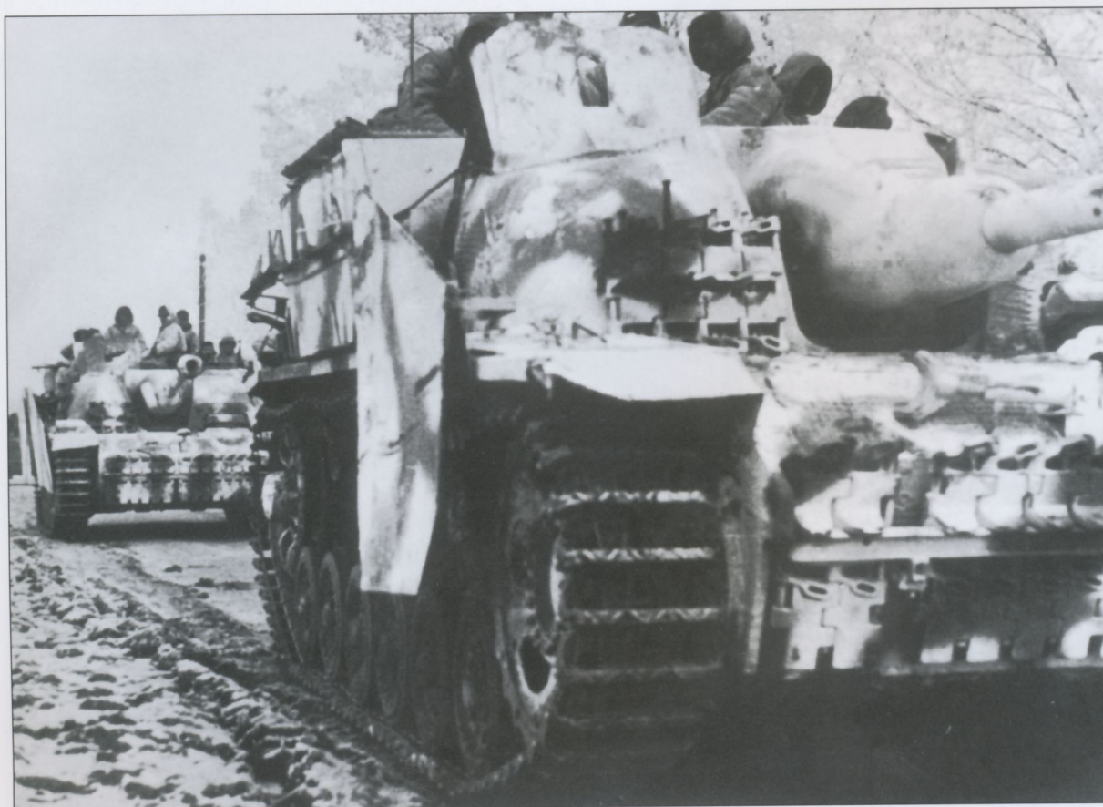
This late StuG.III Ausf.G is fitted with the welded mantlet that has a hole in the upper left side to accommodate a coaxial MG that was introduced in July 1944. Only one piece of Schürzen is left on the right side, illustrating the practicality of the modified hanger system seen in one of the previous photographs. The photograph was taken in Silesia in late March 1945.
