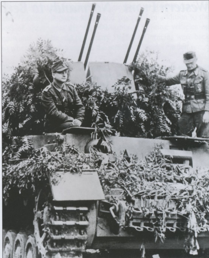
Another new anti-aircraft weapon in the Wehrmacht arsenal, was the 'Wirbelwind' mounting the 2cm Flakvierling 38. The first 17 were completed in July 1944 and, starting in September, began to be issued to the Pz.-Fla-Zug of the Panzer units on the basis of four 'Wirbelwind' and four 'Möbelwagen' each.
