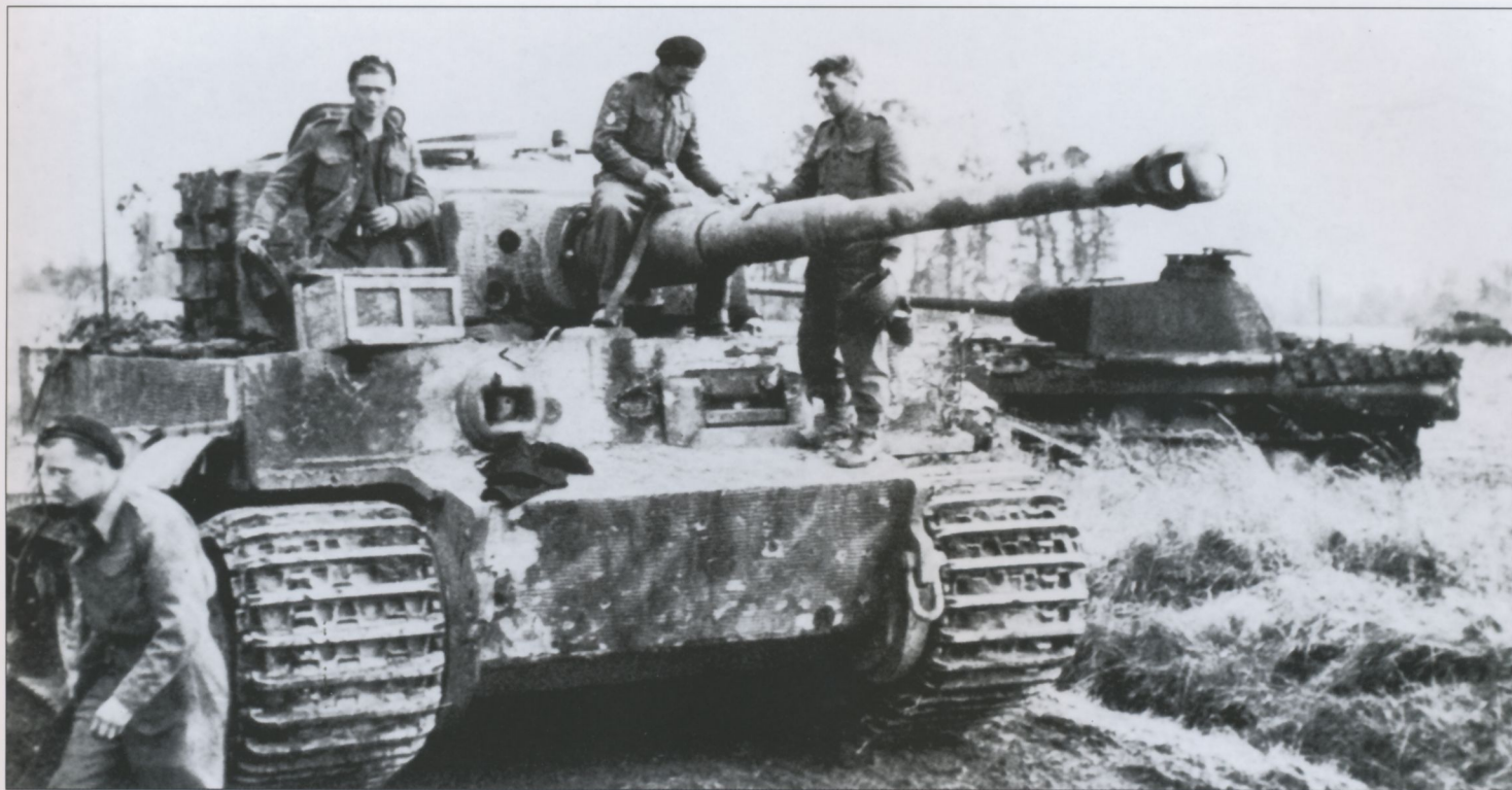
This Tiger I from 1./s.SS-Pz.Abt.101 has been recovered by British soldiers in running condition. The unit insignia can be seen on the left side of the front plate but the 1.Kompanie insignia, a white rhomboid with a script 'S' inside and a '1' beside it, which was painted on the right side of the front plate, has been obliterated during its short time in combat. Note how shell splinters have damaged the Zimmerit coating, leaving the ochre colored Zimmerit highlighted against the undamaged painted areas. In the background can be seen the Panther Ausf.A from 2.Kompanie, 12.SS-Panzer-Division 'Hitlerjugend' with the turret number '204' seen previously.
