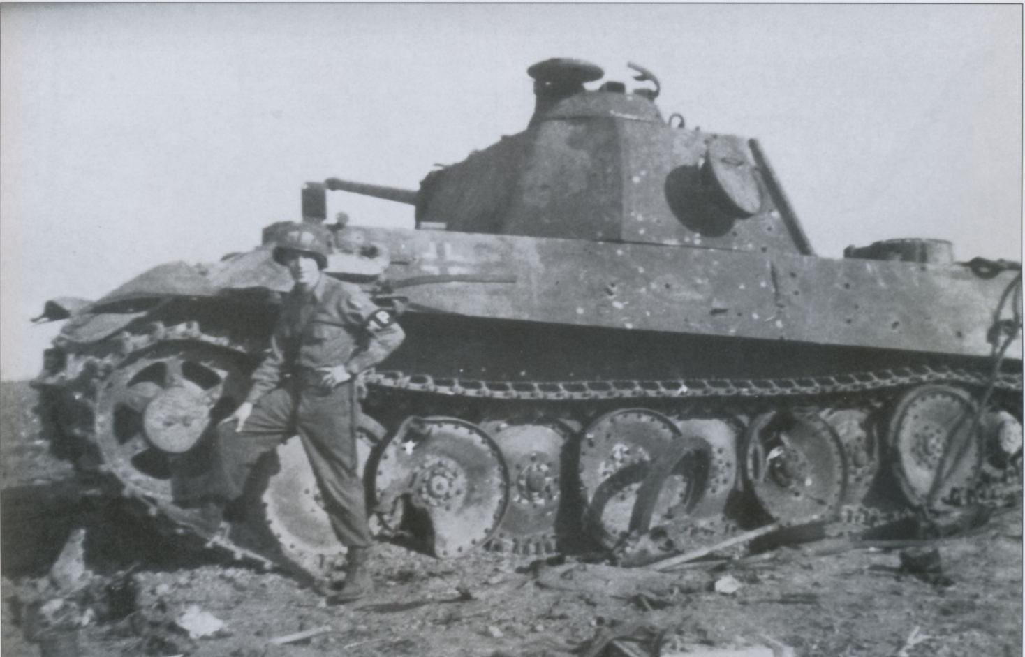
An MP poses beside a badly shot up Panther Ausf.G somewhere in Germany in early 1945. The raised fan tower on the engine deck indicates that this vehicle was fitted with the crew compartment heater introduced in October 1944.
