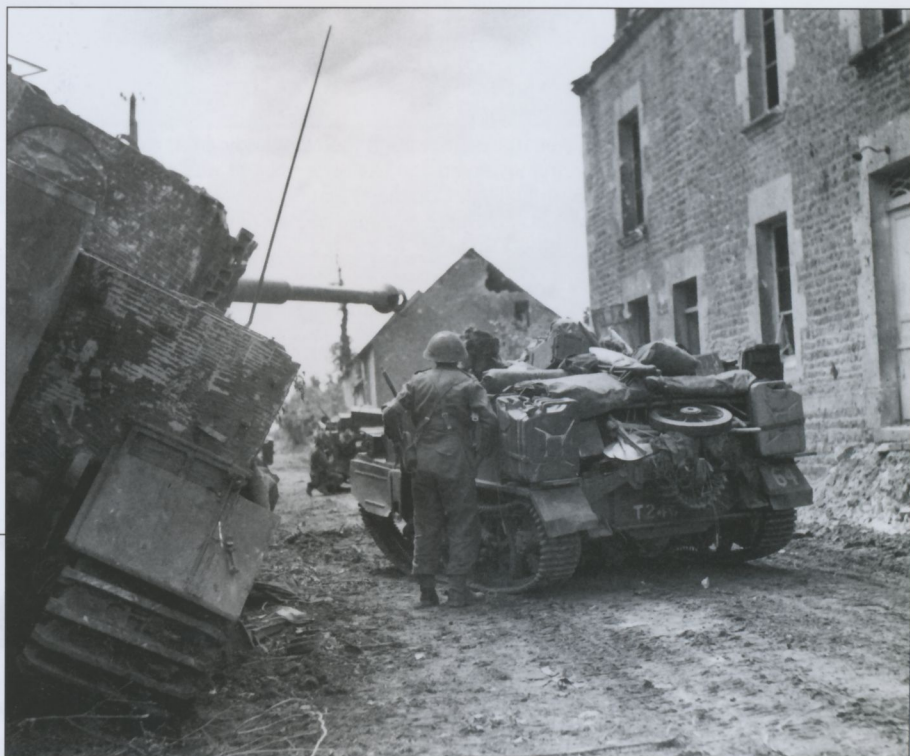
This Tiger I from 1./s.SS-Pz.Abt.101 has been recovered by British soldiers in running condition. The unit insignia can be seen on the left side of the front plate but the 1.Kompanie insignia, a white rhomboid with a script 'S' inside and a '1' beside it, which was painted on the right side of the front plate, has been obliterated during its short time in combat. Note how shell splinters have damaged the Zimmerit coating, leaving the ochre colored Zimmerit highlighted against the undamaged painted areas. In the background can be seen the Panther Ausf.A from 2.Kompanie, 12.SS-Panzer-Division 'Hitlerjugend' with the turret number '204' seen previously.
