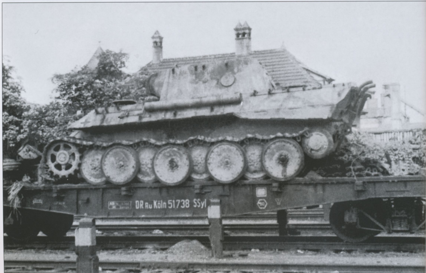
This damaged early Panther Ausf.D was captured in a Czechoslovakian rail yard in May 1945. The commander's cupola, along with the complete gun assembly, is missing. The first outer road wheel has been reinforced with additional rivets between the rim bolts whereas the last three stations still have the original sixteen-bolt configuration.
