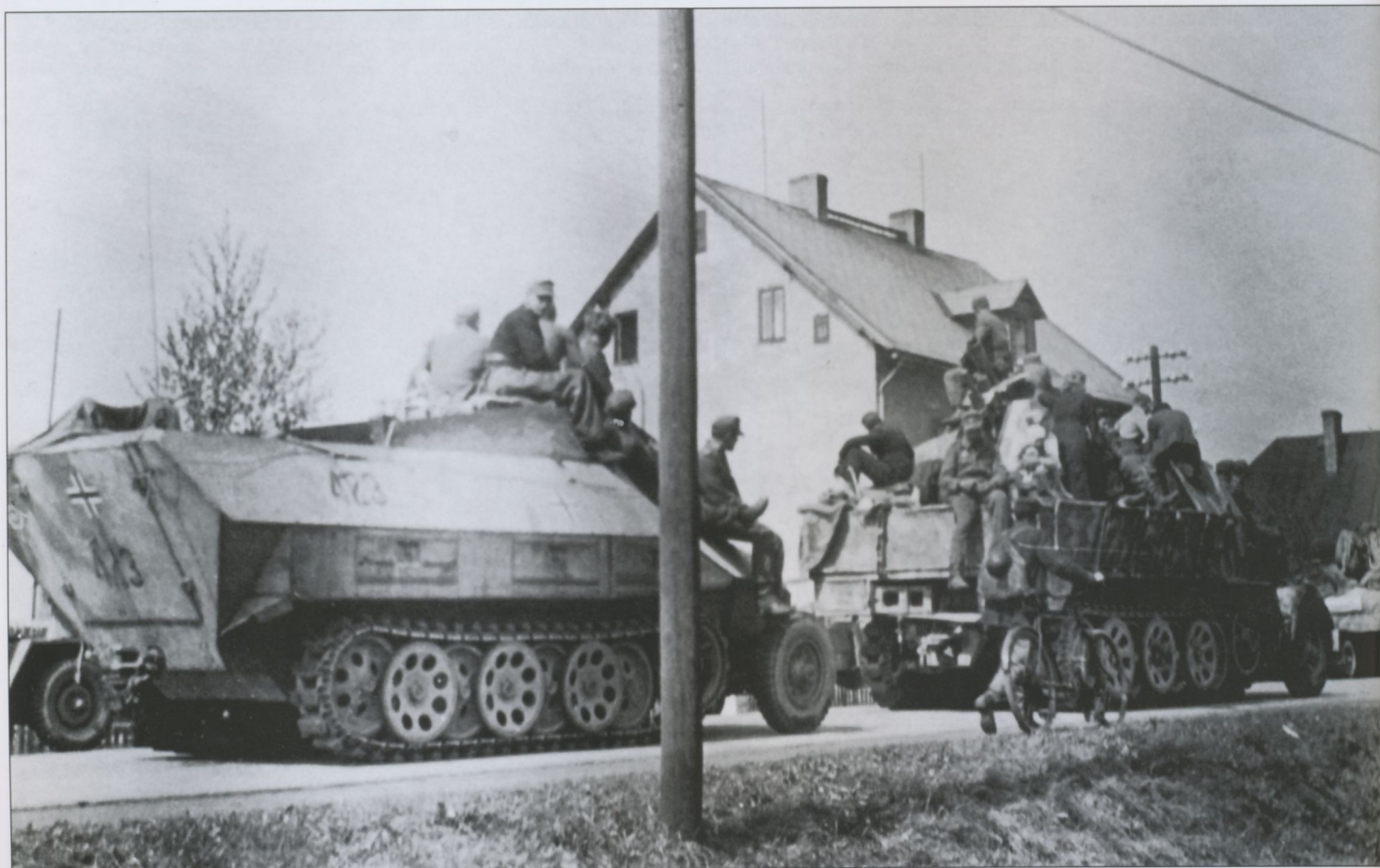
An Sd.Kfz. 251/9 Ausf. D follows an Sd.Kfz. 7/2 into captivity after the cessation of hostilities in 1945. The marking on the left rear of the Sd.Kfz. 251/9 looks like it may be the 'Windhund' emblem of 116. Panzer-Division. The gun barrel of the 3.7cm Flak 43 has been removed, probably to render the weapon inoperable.
