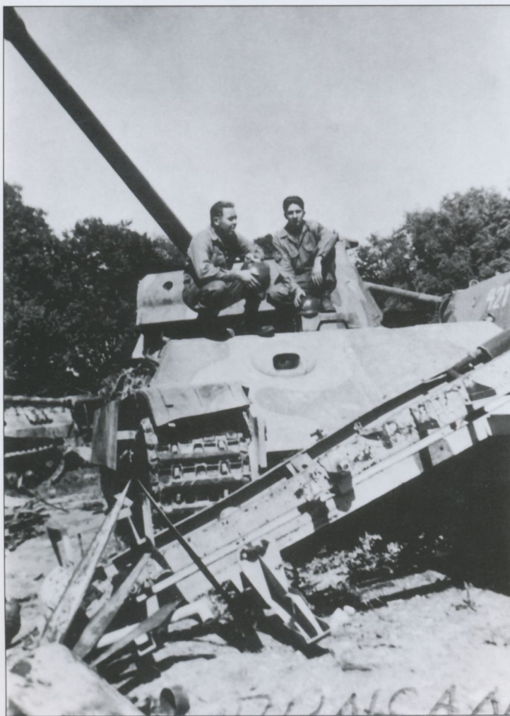
Two U.S. servicemen pose with a Panther Ausf.A near Braunschweig, Germany in early 1945. The penetration hole from the shot that knocked it out can be seen just below the top of the engine deck. The resulting fire has burned away the Zimmerit coating on part of the hull and side of the turret.
