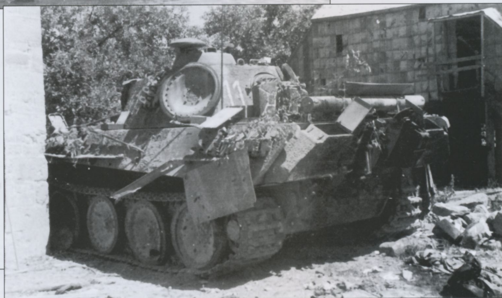
A battle scarred Panther Ausf.G from I./Pz.Rgt.24 of 116.Panzer-Division sits abandoned beside a French café during the late summer of 1944. The Panthers from this unit are noted for carrying spare road wheels bolted to the back of the turret and relocating the gun cleaning rod tube onto the back of the engine deck. Another unique trait is the Jerrycan racks attached to the rear of the hull inside of the rear stowage bins.
